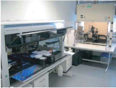
Fig1: For automated sample preparation we offer access to a pipetting robot equipped with a 96 channel pipetting head plus 4 independent channels ("Star" from Hamilton, left) and an automated microarrayer („Pro“, BioRad, right).
