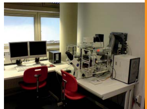
Fig. 2: Here we show one of our automated screening microscopes ("ScanR", Olympus Biosystems) equipped with an incubation chamber for live cell imaging.
